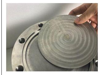
Place the S/S support disc onto the S/S support mesh.
