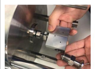
Tilt the extruder to one side, and connect other high pressure connections as left photos shown.
