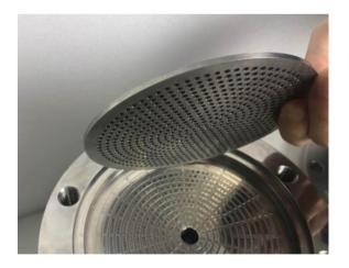
Place the S/S support mesh into the center cavity of the extruder base.
