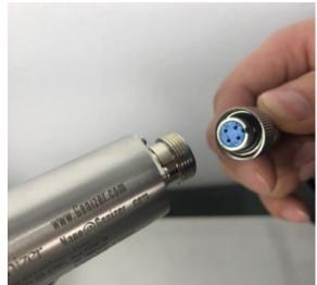
Connect temperature-pressure dual parameter transmitter with TEE.
