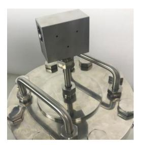
Stand the extruder upright. Connect TEE with another high pressure tubing (Lg. 109MM).
