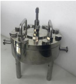
Carefully place required membranes on the S/S support disc, and cover the extruder top, then thread eight cap screws.
