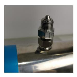
Install the outlet check valve.
