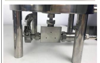
Place the supplied sanitary gasket onto the end of outlet port and connect to the hose barb using Clamp
