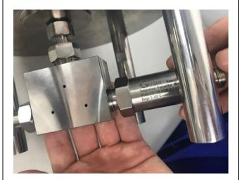
Connect temperature transmitter to TEE.
