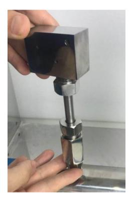
Connect High Pressure Long Nut and Tubing (Lg. 110MM) to the ELBOW.
