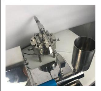
Connect the longest high pressure tubing (Lg. 300MM) to the TEE and ELBOW to link the Nanopump and extruder.
