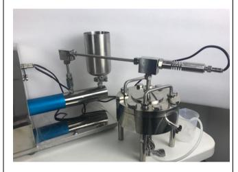
Connect the transmitters' electric code to Nanopump to finish the general assembly procedure.
