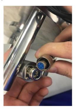
Connect the electric cord with temperature transmitter.
