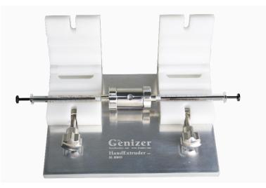
Connect the gas-tight syringe (0.25mL, 0.5mL, 1mL, 2.5mL) in two end
