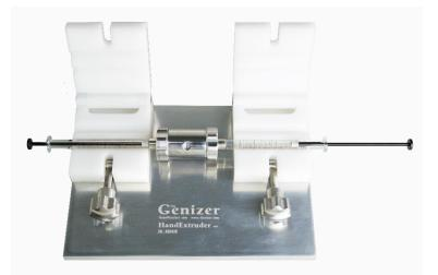
Extruding through 800, 400nm, 200nm, 100nm (if needed 80nm, 50nm, 30nm) nano pore membranes
