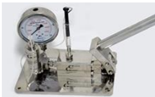
HandPump with Chamber
